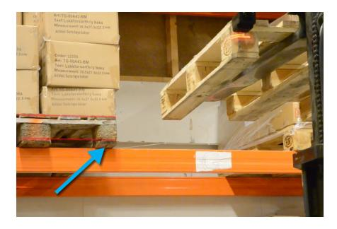
3. Start moving the pallet into place. When pulling back, the upper laser line should be positioned mid-way on the pallet feet. This is a good indicator that it is safe to continue pulling back without the risk of touching the shelf or pallet. If the laser lines converge up or down, the tower is slightly tilted and needs to be corrected first before trying again.
