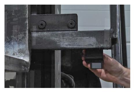
3. Position the mounting adapter as far to the left side of the carriage as possible, to maximize laser coverage. However, when the unit is mounted, it should not protrude to the side of the carriage.
