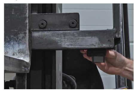
4. After the adapter is attached and leveled to the carriage, continue by holding the RedEye-unit right side up and slide it on the adapter. The bottom magnet on the adapter bounds with a metal plate inside the unit and keeps it securely mounted.
