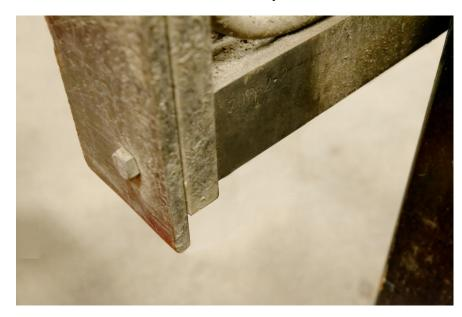
2. Hold the suitable adapter with the top magnet turned up and mount it on the rear edge of the steel beam. The two magnets guides the adapter into position - make sure it is seated all the way! The magnets keeps the adapter secured even through heavy vibrations and bumps.
