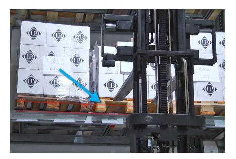
3. Lift the pallet as normal and pick the pallet from the shelf, and lower the carriage. The pallet is now safely fetched.
