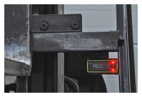
5. When the adapter and unit are installed properly, the upper laser line (that is emitted on to a surface) should illuminate appoximately mid-way on the side of the left fork. If it does not, the unit is either
